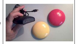
The SimplyWorks® Switches shown here is a low profile, large diameter wireless switch that can be used with any of the SimplyWorks® receivers to give switch, mouse, or keyboard functions.
